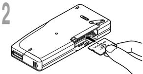
2 **Face the card the correct way and insert it into the card slot as shown in the diagram.**
