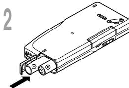
2 Insert two AAA batteries, observing the correct polarity.
