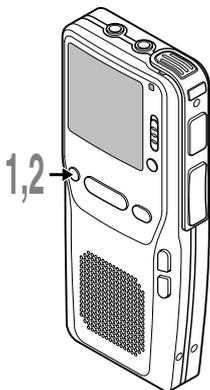
**1** Select any file in the folder, then press and hold the **ERASE** button for **3 seconds or longer**.
