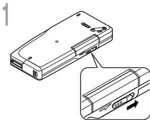
1 **Slide the card cover lock in the direction indicated by the arrow.**
