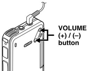
It is possible to monitor your recording by listening to the recording while recording is in progress. Insert the earphone plug into the earphone jack and use the VOLUME button to control the volume level.
