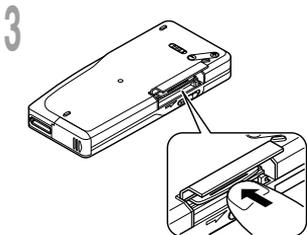
3 **Push the card inward to unlock it, and let it eject partially.**
