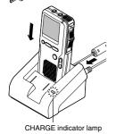
Turn ON the recorder and, remaining the slide switch at the **STOP** position, set it vertically in the cradle.
